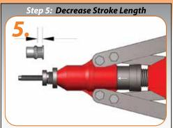
To adjust the stroke to suit thicker walled materials screw the stroke adjusting nut. When in the desired position lock in place using the stroke adjustment locking nut.
