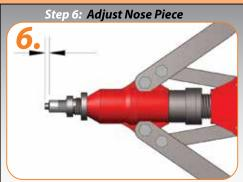
Adjust the nose piece so that the unthreaded tip of the mandrel protrudes from the end of the blind nut rivet when it is threaded on. Lock in place using the nose piece locking nut.
