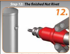
The nut rivet should now be securely in place and unable to turn. This will give you an extremely strong fixing thread for your required application.
