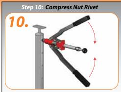
Push the tool lever handles inwards to compress the nut rivet against the wall of the tube. This will fasten the nut rivet in place.
