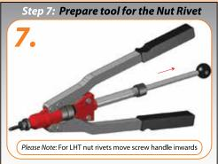
Prepare the tool for the nut rivet insertion by opening the handle levers and moving the screw handle outward. Moving the screw  $\,$ handle outward will rotate the mandrel anti clockwise.
