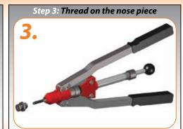
Thread the nose on to the main body of the tool. The nose piece being used must match the size of mandrel being used. Ensure the nose piece locking nut is on the nose piece before threading on.
