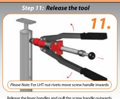
Release the lever handles and pull the screw handle outwards This will unthread the mandrel from the nut rivet.
