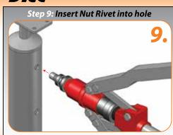
With the nut rivet on the mandrel of the tool insert the nut rivet in to the pre-drilled hole.
