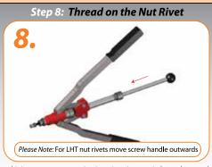
Hold the nut rivet against the thread on the mandrel. Simultaneously push the screw handle inwards. Pushing the screw handle inwards  $% \left( 1\right) =\left( 1\right) \left( 1\right) \left($ will thread the nut rivet on to the mandrel.
